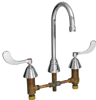
#05508 (785-CP) • 8" Centers • Concealed Fitting • 4" Blade Handles • 3-1/2" Rigid/Swing Gooseneck Spout (GN1A)
