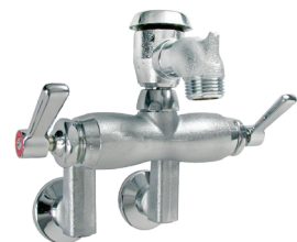
#55130 (305-VBRRCF) • Vacuum breaker spout short • 3/4" Hose thread outlet • Pail hook • Adjustable from 4" to 8-3/8" centers • With integral stops
